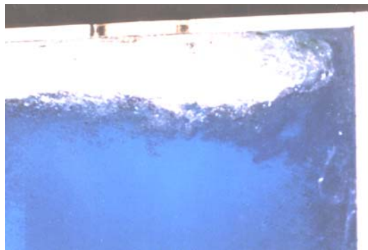
Fig. 3 Formation of bubbles before and after side-wall impact: SNU model, 30% filling. (a) Before impact (b) After impact and wave run-up
